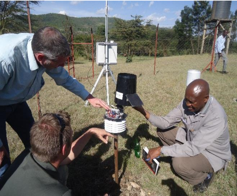
c) Inspecting the Tilting bucket of Rainfall one low cost equipment being experimented Bomet courtesy of MAMASE
